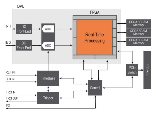
Figure 1. Simplified block diagram of the U5310A PCle ADC card, with on-board real-time processing.
