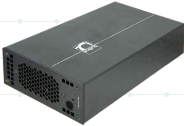
Figure 6. The SA230E is a fully shielded module, maximizing both ESD and EMI protection.
