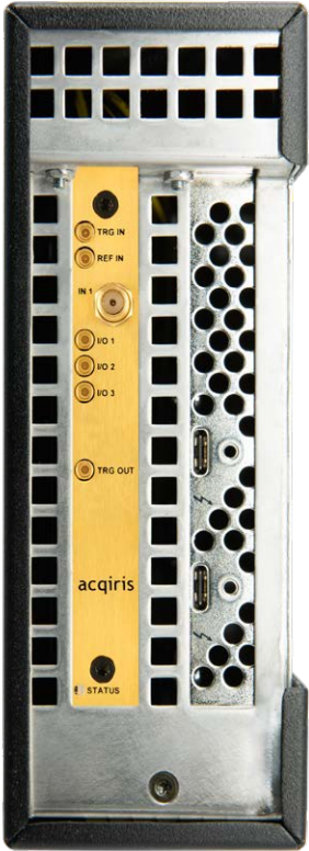
Figure 3. SA230E signal connectors, with analog inputs and multiple programmable I/O signals.
